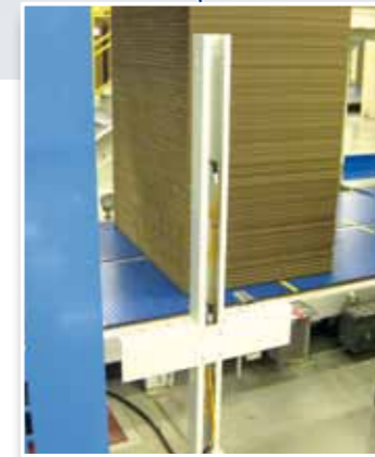
Entrance control For save working near the exit conveyor.
