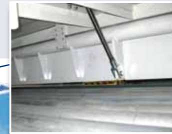
Lift / trapdoor A laser-controlled heavy duty lift with a trapdoor for pallets or (optional) waste sheets.
