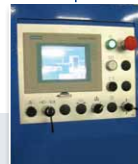
Main control panel With an integrated touch screen.
