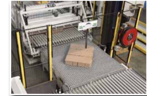
Ball table (patented) Turning of multiple bundles simultaneously
