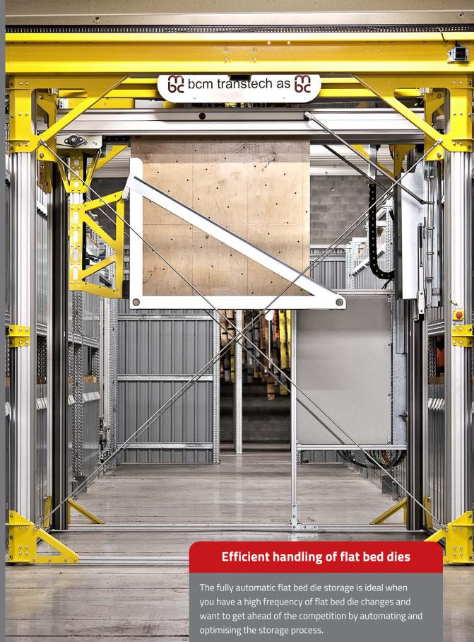
Specifically, it lets you run a high volume storage with few operators, because the storage unloads and loads the transport trolleys, while the operators can solve other tasks. In addition, the storage keeps track of the flat bed dies, so that it is easy to locate them.
