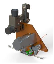
RTM Application Head – Applies the rippa tape on defined place on product with defined length.Position and length of silicone tape on product is defined by user on HMI panel
