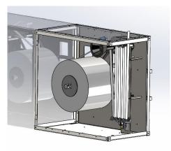
STM unwinder – Unwinds, stores and feed the Silicone tape to the application head. Unwinder for Jumbo spool and pancake rolls 2. STM Application Head
